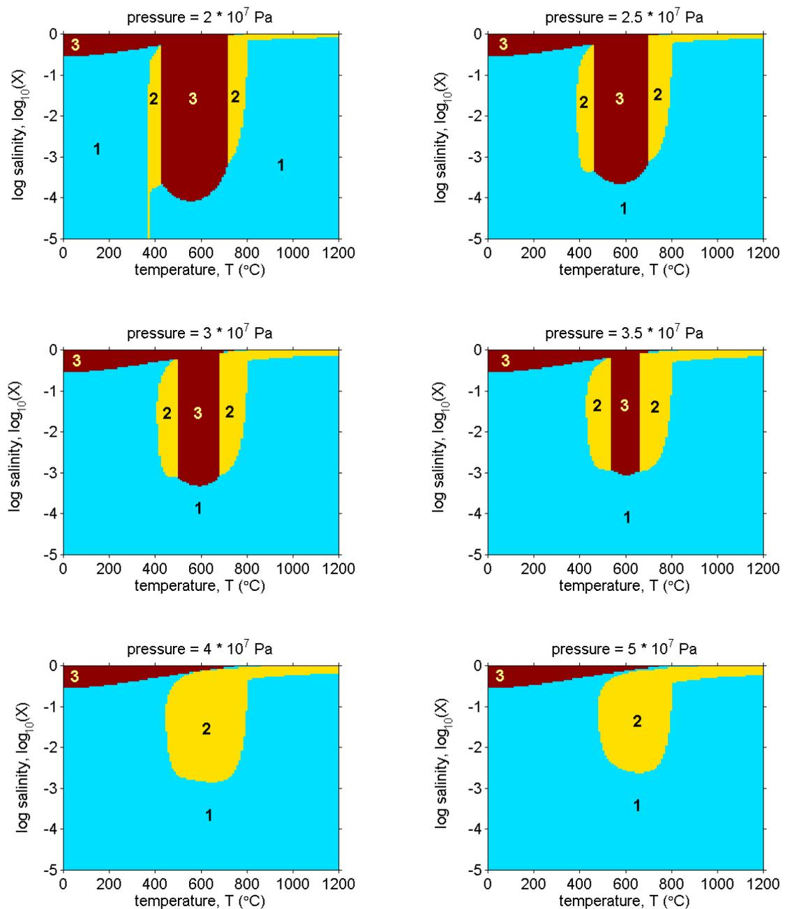
**Figure 7.1:** Isobaric cross-sections of the H<sub>2</sub>O-NaCl state space for a range of seafloor pressures ( $10^7$  Pa corresponds to a depth 1 km below sea level). Regions of state space are labelled as follows: **(1)** – Unsaturated single phase fluid. **(2)** – Unsaturated two-phase fluid (liquid + gas). **(3)** – Saturated single-phase fluid. Thermodynamic data from Palliser & McKibbin (1998a).
