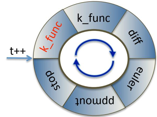
In our simple script, the first instance of the `k_func` device has a program that executes only once per timestep. It assigns value `1` to k-variable `begin` if the timestep counter `t=0` (otherwise assigns `0`), then assigns `1` to k-variable `output` if `t` is divisible by `100` (otherwise `0`), and then assigns `1` to k-variable `end` if `t` equals or exceeds `2000`. NB these k-variables are defined by `def` commands before used.
