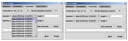
Fix the length of pipe of type 1. The program will automatically compute the length of the type-2 pipe by simple difference. Don't forget to click on "Add constraint" to validate the choice. You may repeat the operation to handle several constraints. You may also delete constraints.
