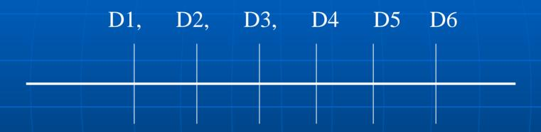
D1 >= D2 >= D3, D4 <= D5 <= D6Fixed at six diameters, five sections
