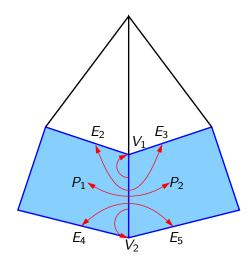
Back-pointers from  $V_1$ ,  $V_2$ ,  $P_1$  and  $P_2$  to one of their edges.
